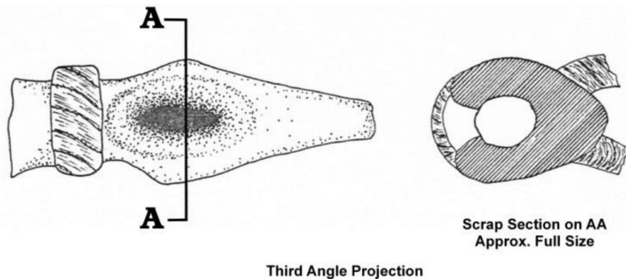
Figure 5.45: Side-Blown Instrument Blowing Apertures
