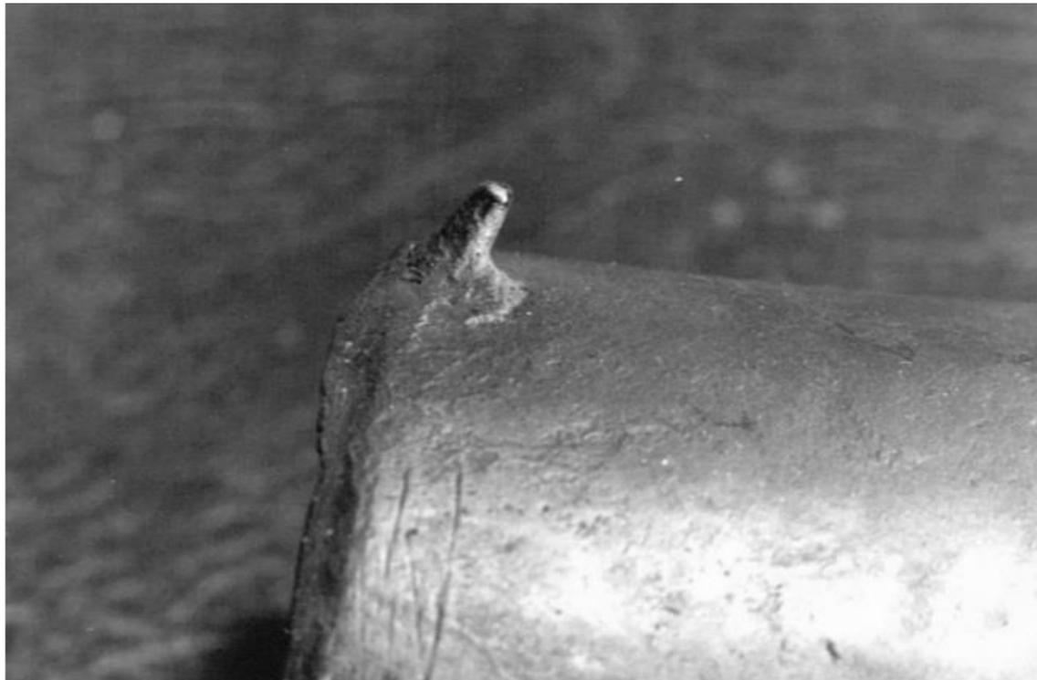
Plate 5.25a: A Cast-on Spike
