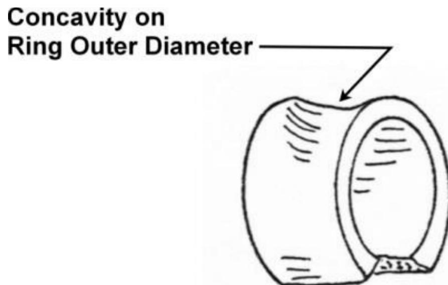
Figure 5.34: Sheet Metal Ring Mount Form
