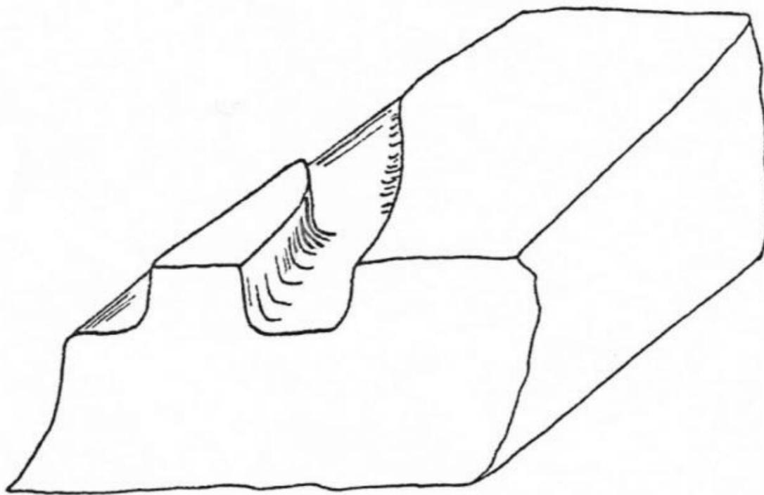
Figure 5.28: Creating an Integral Carrying Loop
