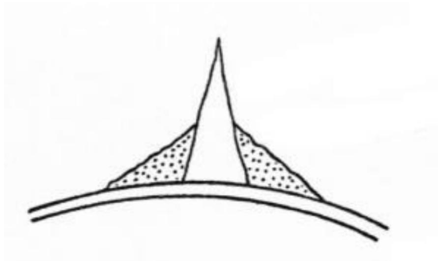
Figure 5.39: A Cast-On Spike on SD14K
