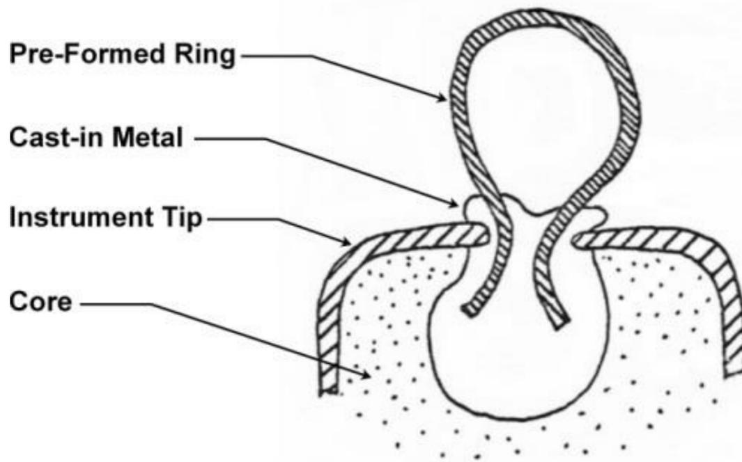
Figure 5.35: A Wrought Cast-in Ring Mount
