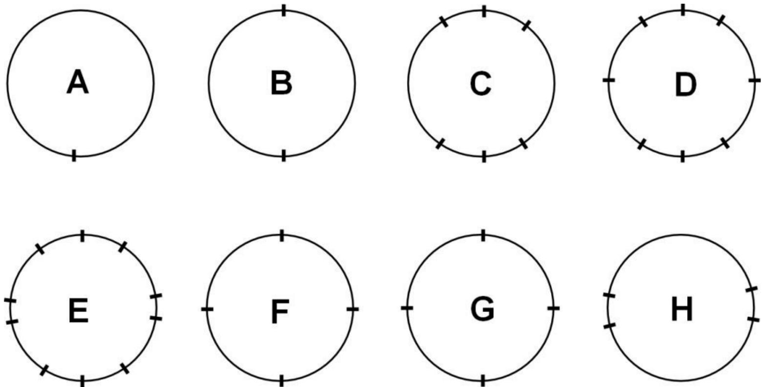
Figure 5.20: Different Chaplet Configurations
