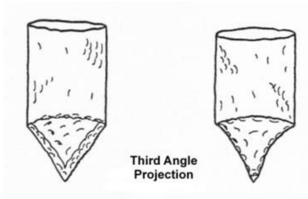
Figure 5.41: Possible Designs of the Drill Bit
