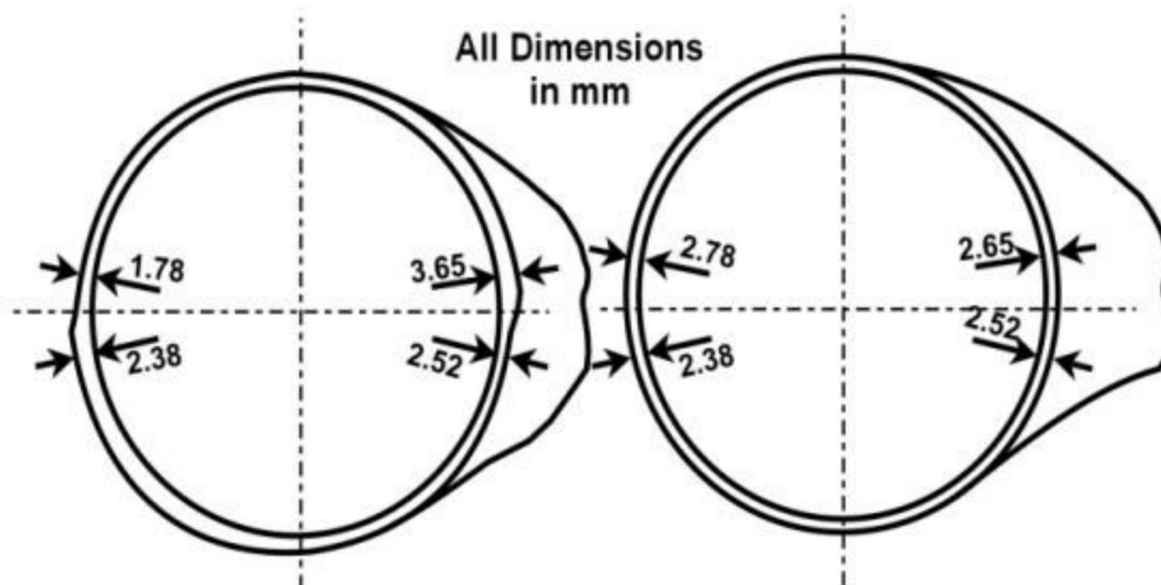
Figure 5.26: Measured Wall Thicknesses on SD19A
