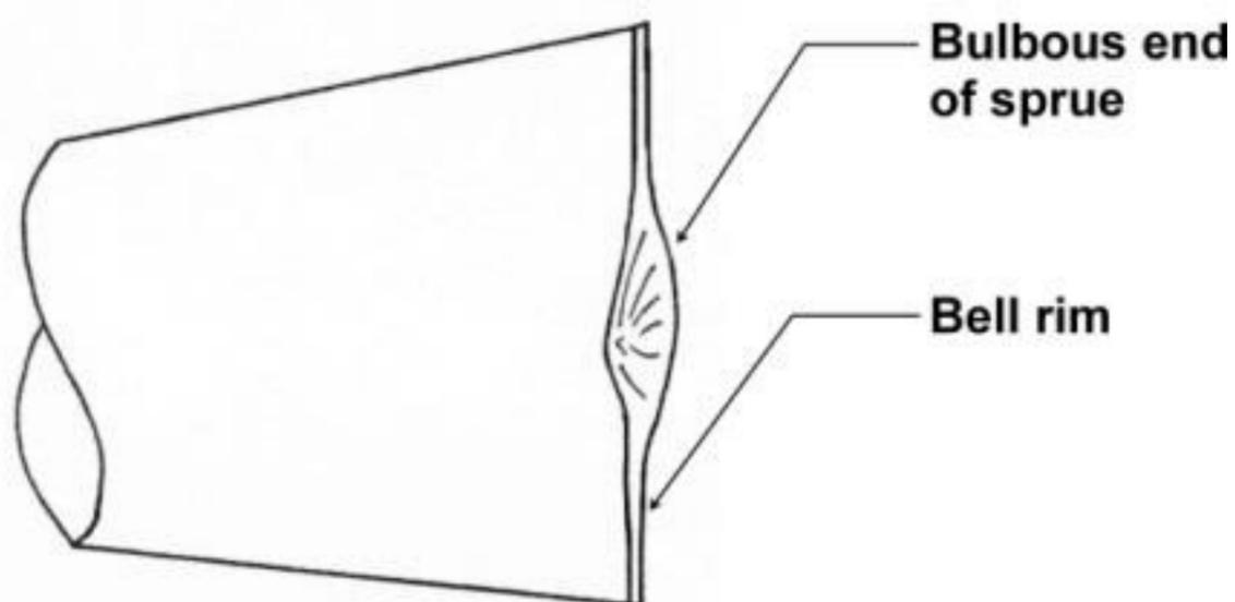
Figure 5.10: An Abraded-back Sprue Ending
