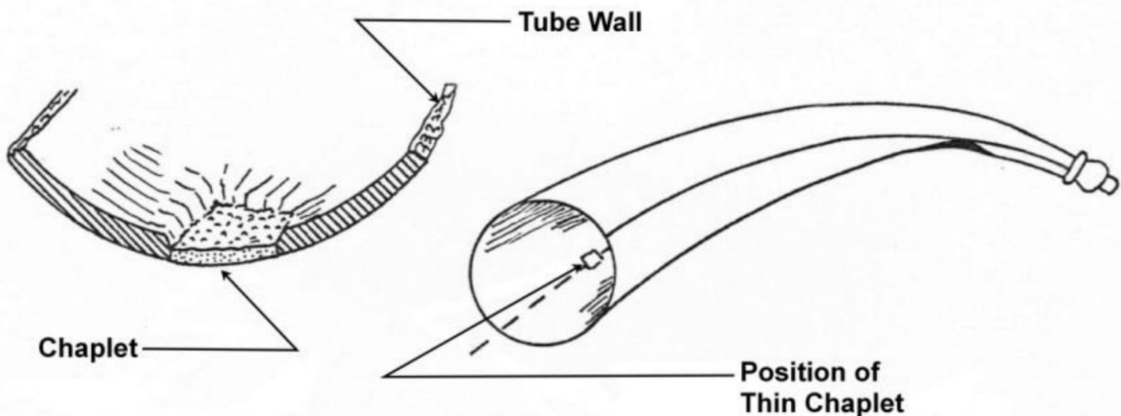
Figure 5.3 Surface Chaplets in a Tube Wall
