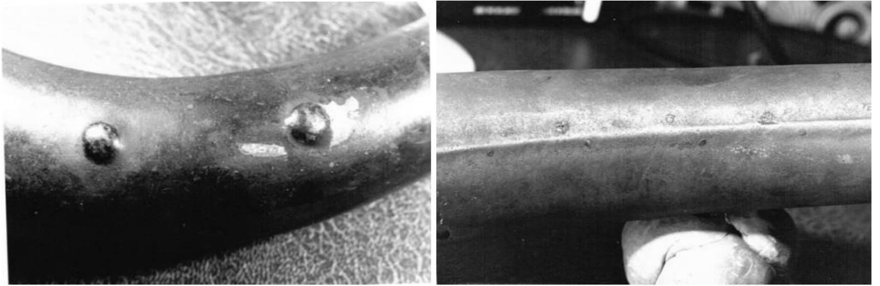
Plate 5.12: Chaplet Evidence on Tube Walls
