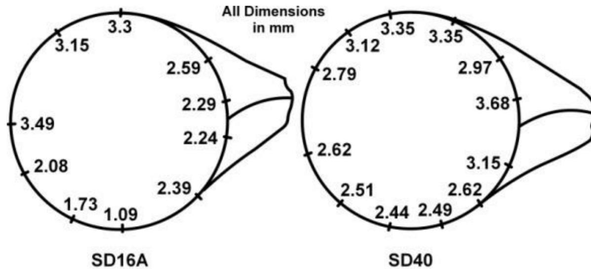
Figure 5.25: Measured Wall Thicknesses on SD16A and SD40
