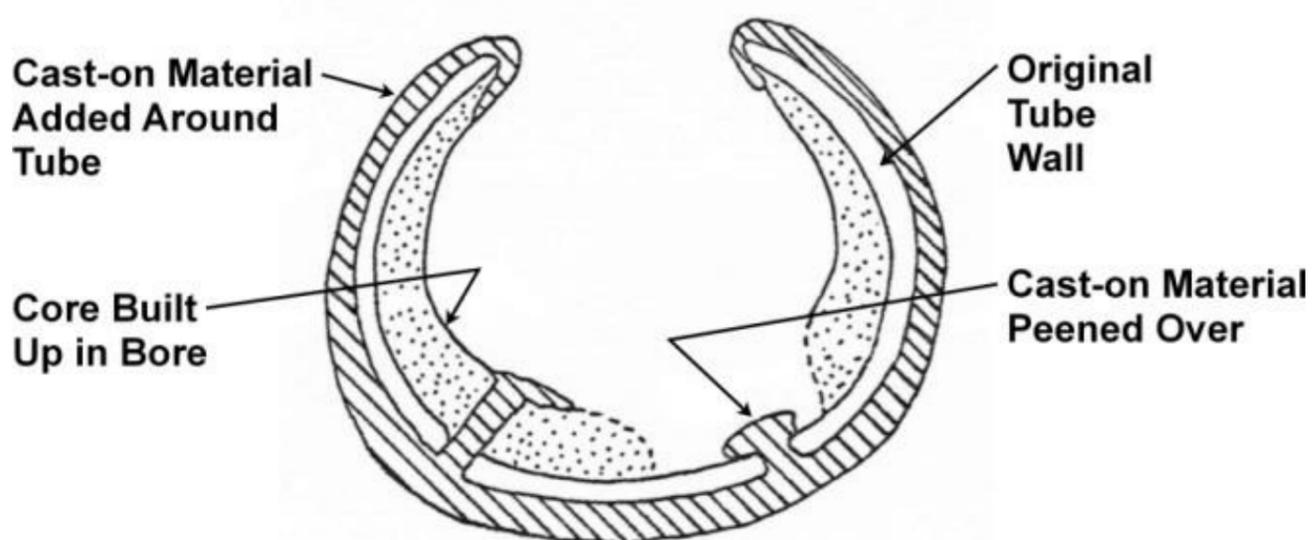
Figure 5.37: A Cast-on Tube Repair
