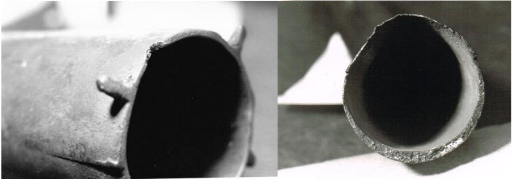
Plate 5.10: Registration Errors on Bell Ends
