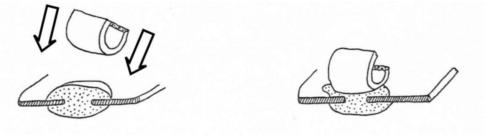
Figure 5.33: Attaching Tube Ring Mounts
