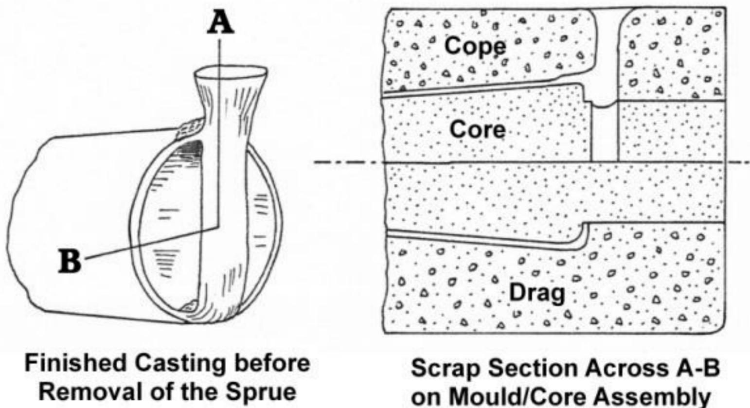
Figure 5.11: Feeding the Casting
