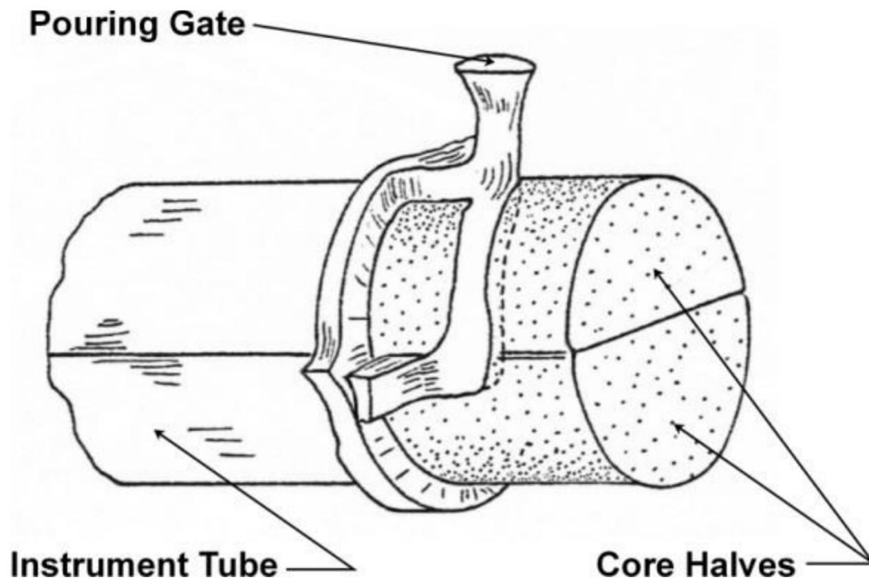
Figure 5.12:Gating Evidence on Bell Ends
