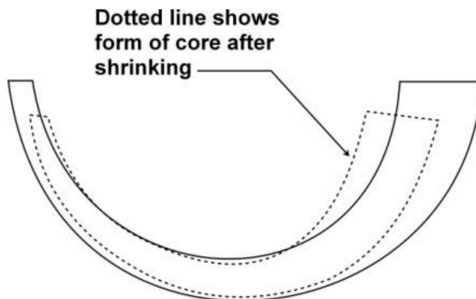
Figure 5.7: The Shape of a Core after Shrinking
