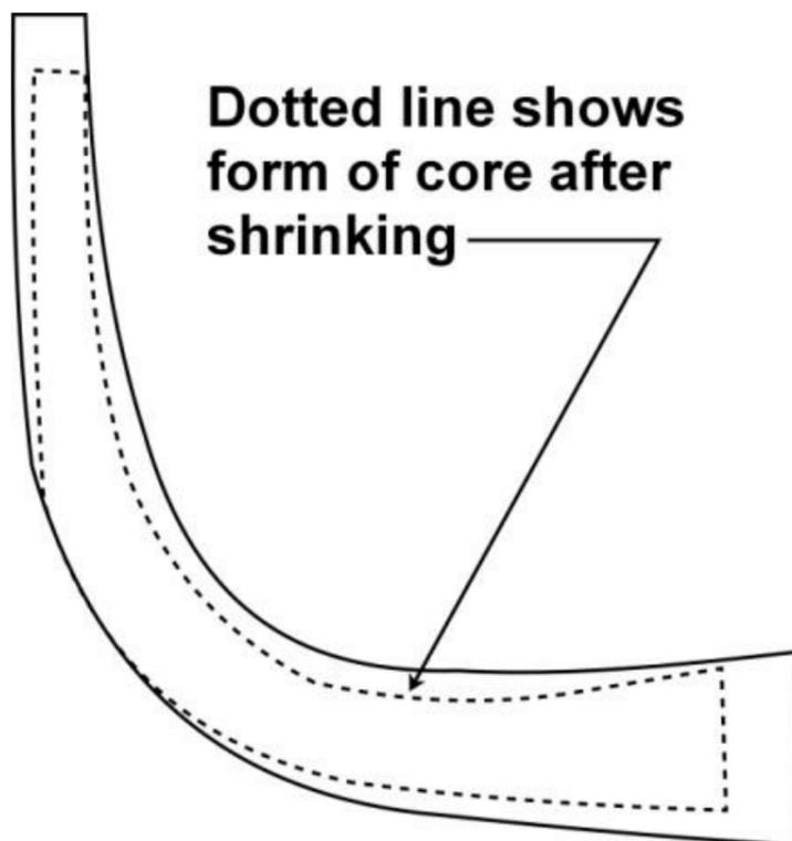
Figure 5.8(a): A Further Core Shrinkage Pattern
