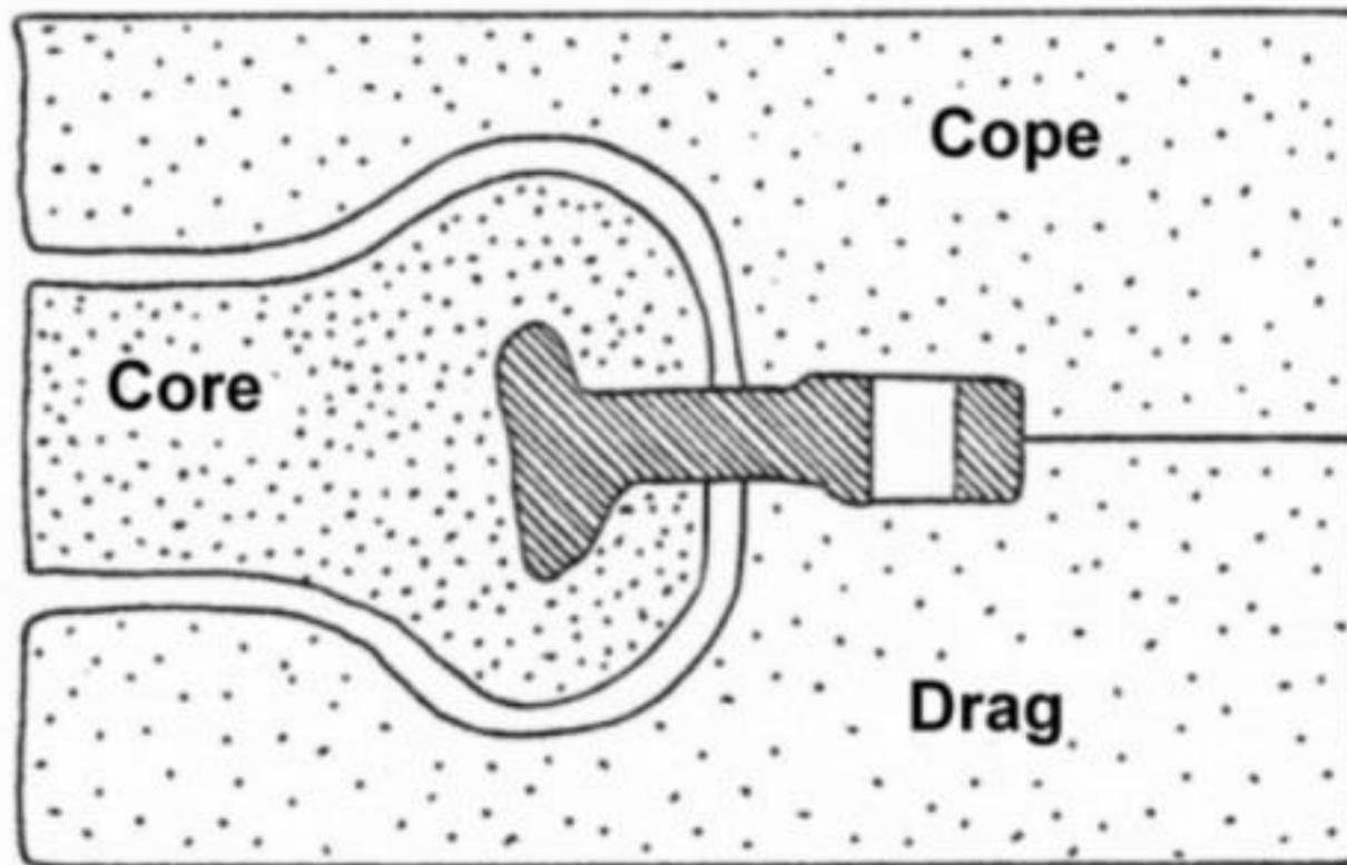
Figure 5.32: Casting in a Tip Ring Mount
