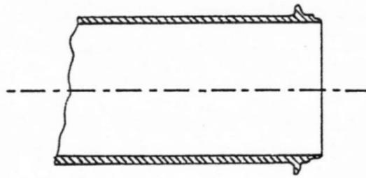
Figure: 5.5: A Bell-end Cross-Section
