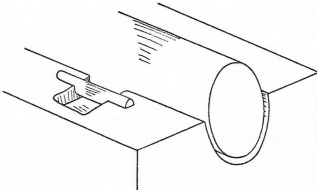
Figure 5.30: A Cored-out Carrying Loop
